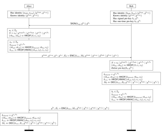
Figure 2: SP, a variant of Signal with minor differences. Alice requests a signed pre-key from Bob (via the server) and sends an initial message  $M_0$ . Bob accomplishes his side of the key exchange and obtains  $M_0$ . Bob later sends his reply  $M_1$ , illustrating the Axolotl ratchet post-AKE. We ignore the hash-based ratchet that occurs when two consecutive messages are sent in the same direction.  $c_i$  refers to various constants found throughout the protocol.
